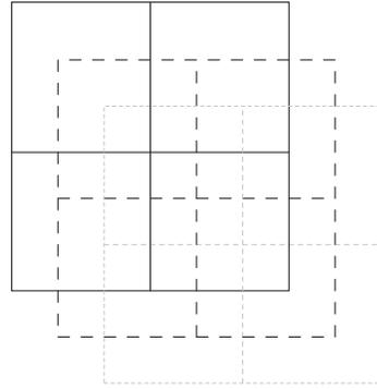
Fig. 2. Tile structure for a CMAC with three layers, and four tiles per layer.
